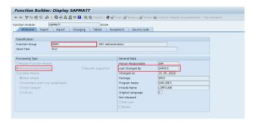
Fig. 26. Properties of Injected ABAP Function Module in Transaction SE37.
