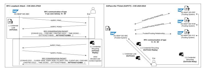
Fig. 15. High-Level Concept of RFC Loopback Attack (left) and SAPass-the-TTicket Attack (right)
