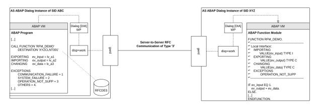
Fig. 2. ABAP Function Module Call via Server-to-Server RFC Communication of Type '3' (modified taken from [10]).
