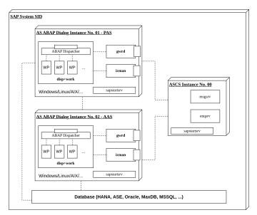
Fig. 1. Simplified Platform Reference Architecture (modified taken from [6]).
